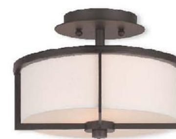
51072-07 CEILING MOUNT 11" DIA 8" H MAX WATT 2 - 40W MED BASE CANOPY 4.75" D WITH BOTTOM SATIN OPAL GLASS DIFFUSER SUITABLE FOR DAMP LOCATIONS
