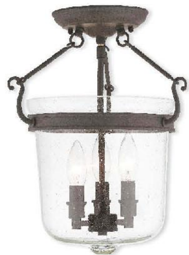
50493-07 CEILING MOUNT 12" DIA 14.75" H CANOPY 6"D MAX WATT 3 - 60W CAND BASE SUITABLE FOR DAMP LOCATIONS
